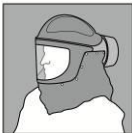
(C) Powered, air-purifying, ventilated respirator
