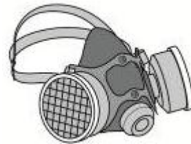
Figure 6: Half-face, particulate filter (cartridge) respirator.
