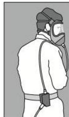
Figure 10: Full-face, positive pressure demand air-line respirator.
